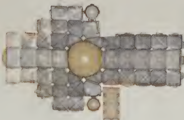
FIG 10 Reflected ceiling plan of the Duomo di Siena (Santa Maria Assunta), Siena (13th century). Drawing by author.
