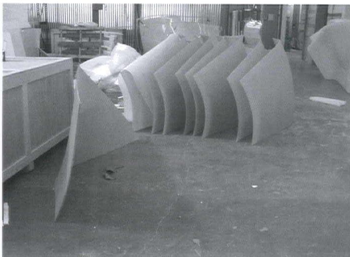
Graft Architects, Tangerine Bar, Los Angeles Left to right: original floor plan; original fiberglass tests using 15' tall interlocking panels; series of final polycarbonate heat-formed panels; revised canopy design using 15 compound curved molds;
