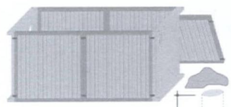
3:30 8. Attach panels to pallets; excavate for privy.
