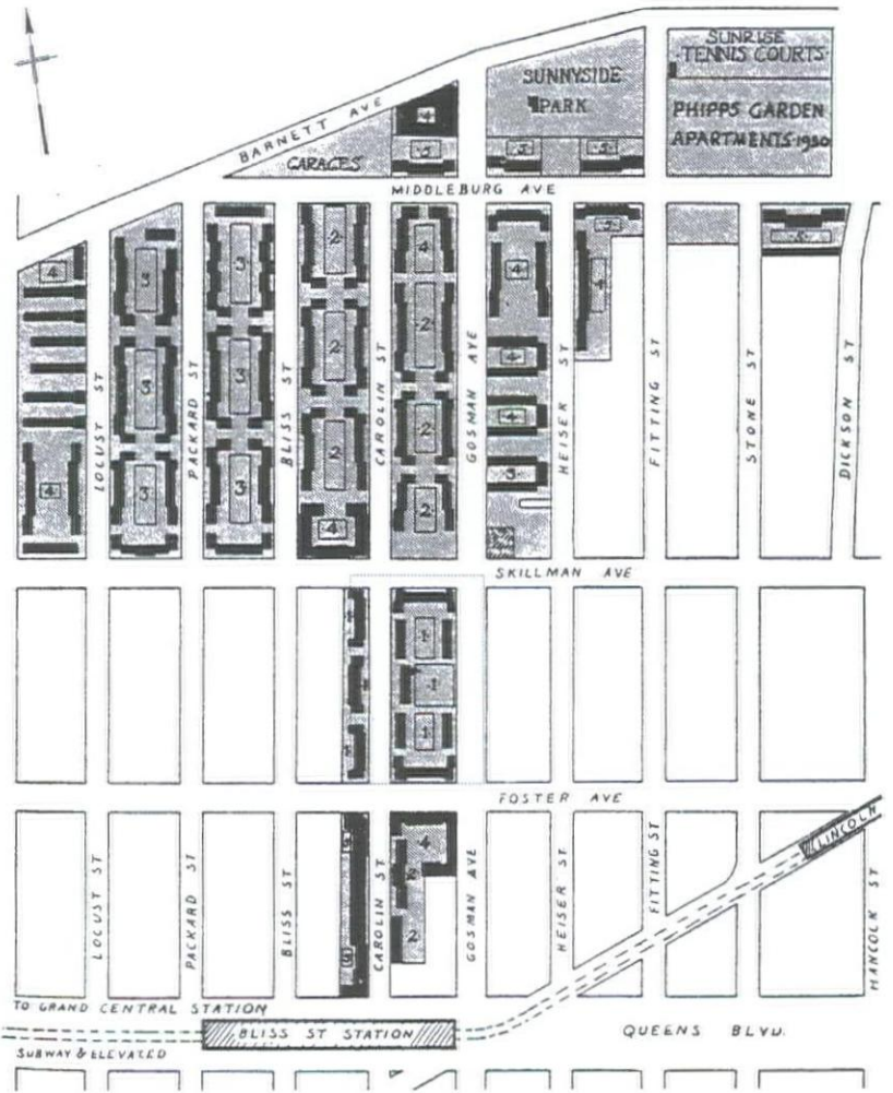
Site plan showing successive building stages: 1 = built 1924, 2 = 1925, 3 = 1926, 4 = 1927, 5 = 1928
