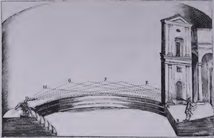
◊ 2. Mario Bettini, acoustical diagram of an elliptical theater (1642). The Baroque strategy of focusing sonic “rays” was an important precursor to the modern theory of reverberation.
