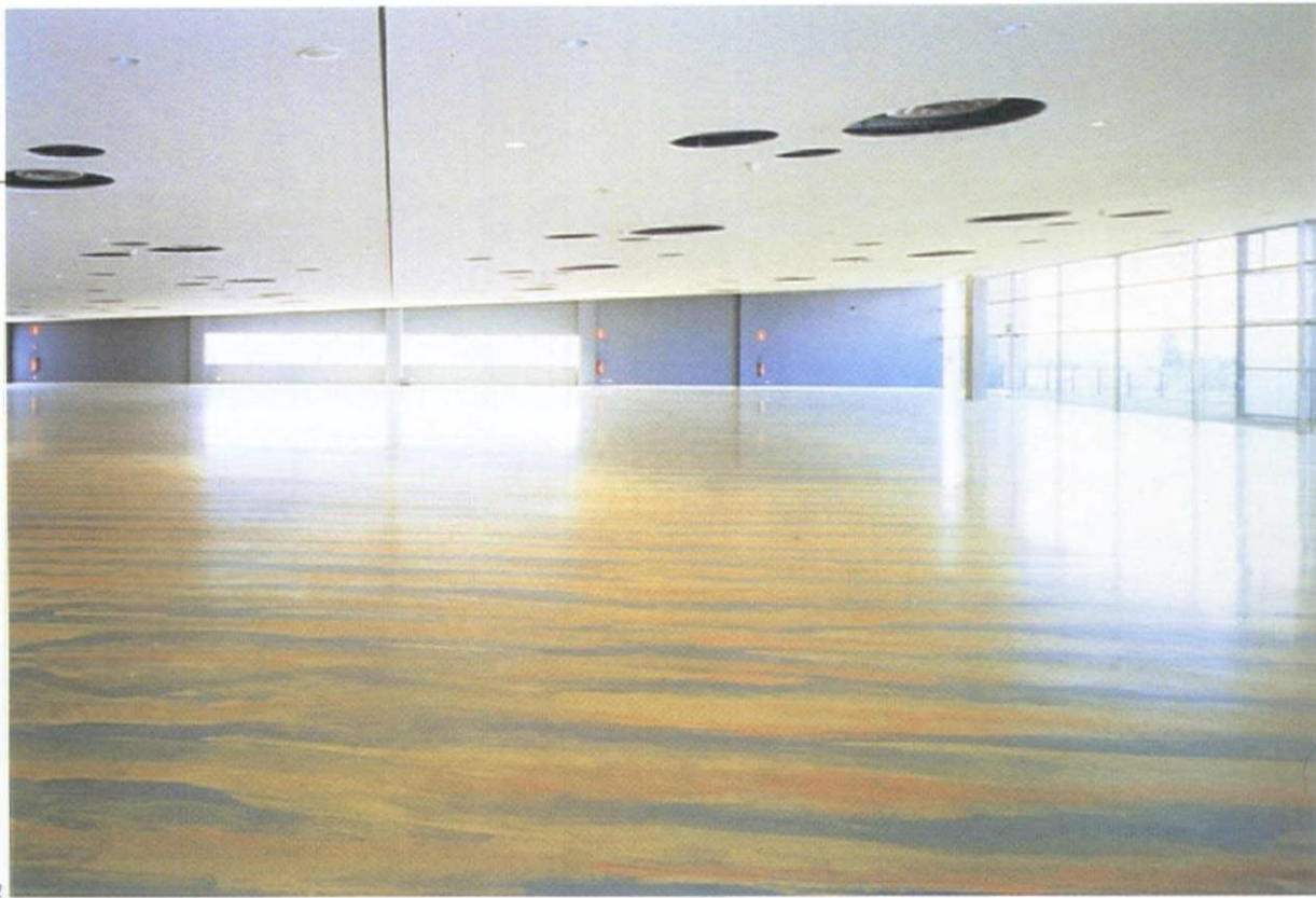
2: The rubber used in the floor of Rem Koolhaas's design of the banquet space of the Lille Grand Palais was poured in place
