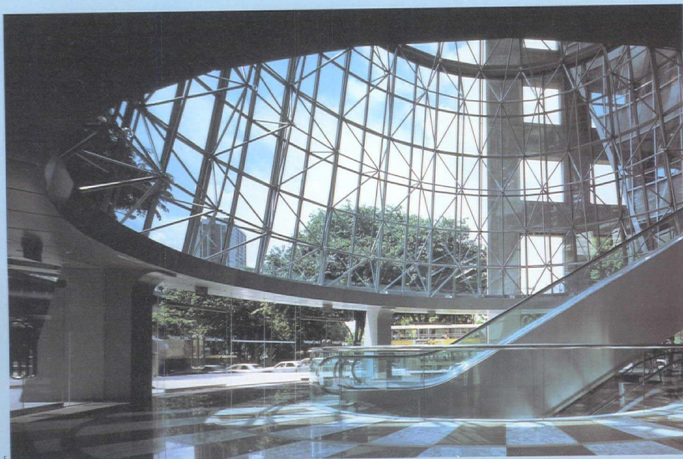
5: Main entrance and atrium. The curtain wall is inclined outwards, reducing solar gains, and creating an intermediate zone between the street and the commercial interior
