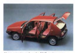
Above, experimental car for FIAT, testing a new structural system. The ideas generated in the design of this car were later partly incorporated in the current Fiat Tipo.
