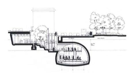
Section through underground station at Piazza Principe on the harbour front, Genoa. The station makes use of the traditionally redundant space below the 'supraelevata' motorway that courses through this sensitive historic district.
