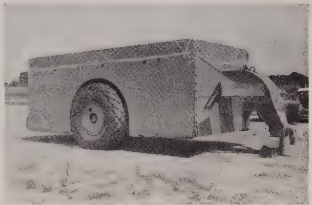
Heavy compaction —This 50-ton rubber tire roller was used to proof-roll the subgrade. The aggregate base was proof-rolled with a 25-ton pneumatic tire roller exerting 82 psi contact pressure.
