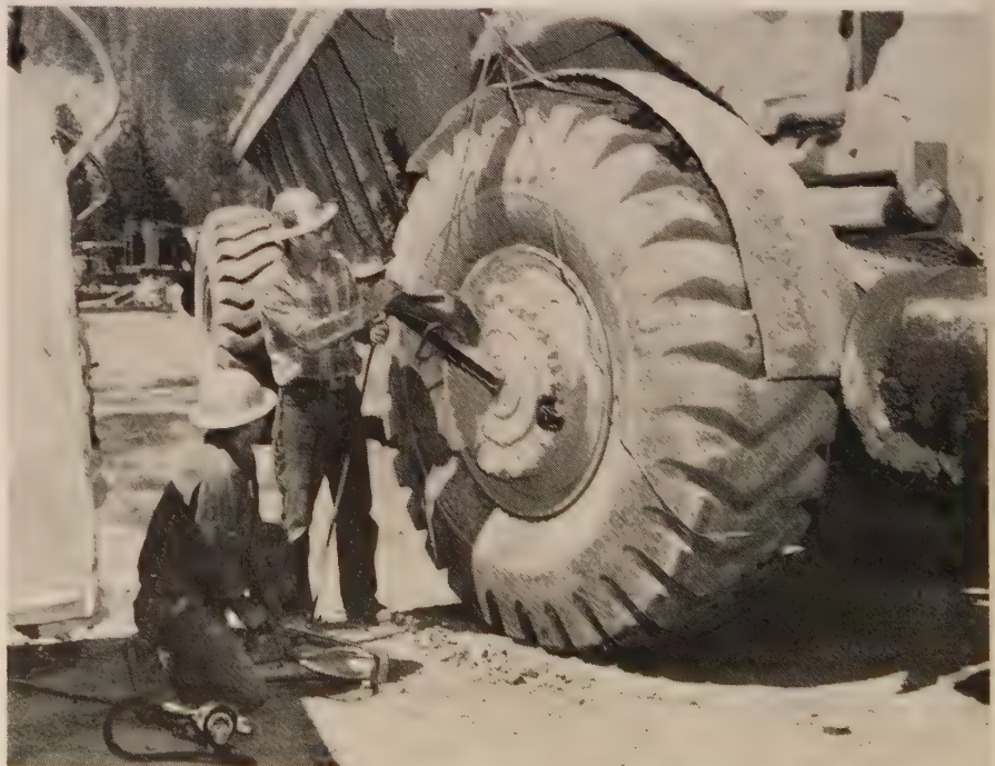
MODERN tire handling equipment enables B. F. Goodrich tire servicemen to handle huge 27.00-33 tires with minimum effort. Large equipment working at Cougar Dam often pauses in front of the service shop to make certain all tires are in good condition.
