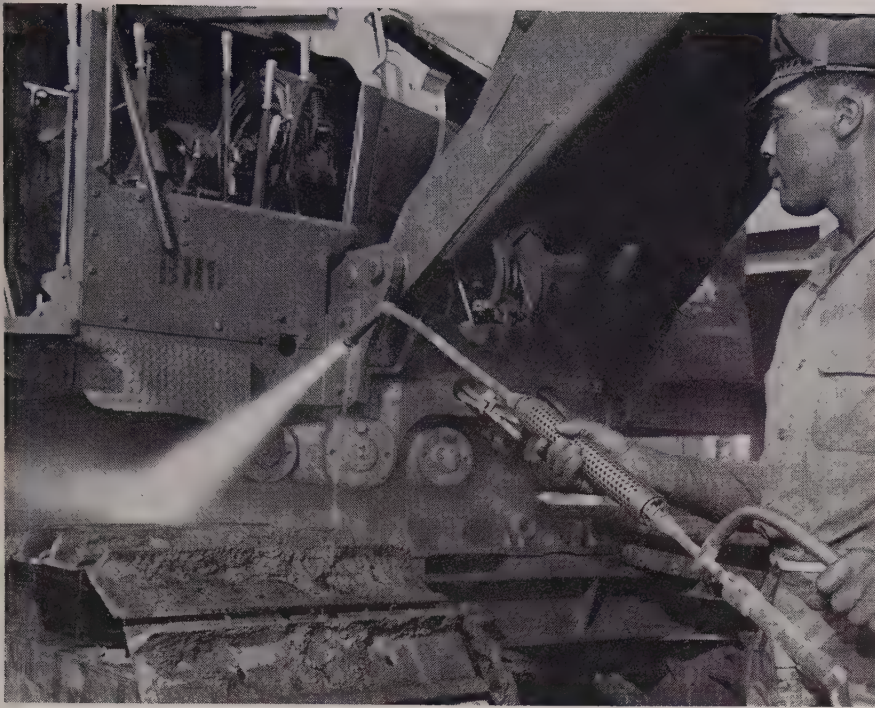
CLEANING is not only a shop procedure prior to overhaul, but is equally important on the job. For example, a high-pressure cleaner mounted on the lube truck can reduce the time of the mechanic during inspection, and the time of the welder in making repairs.
