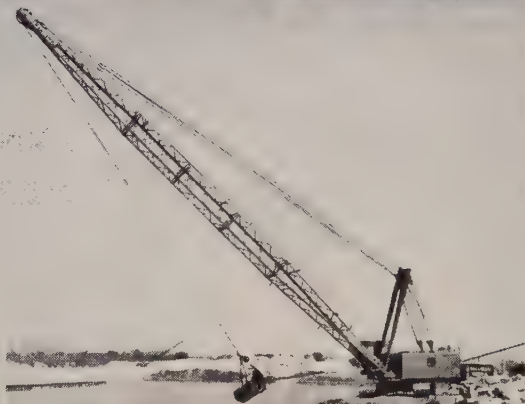
Manitowoc 4500 Vicon dragline dredges 375 yds. of mud and rock per hour.
