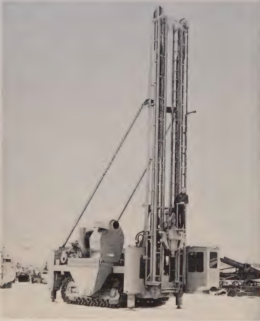
WORKMAN stands on platform mounted on floating rotary head. Picture was taken in manufacturer's yard during assembly. Note hydraulic leveling jacks and pipe for dust-removal hose.
