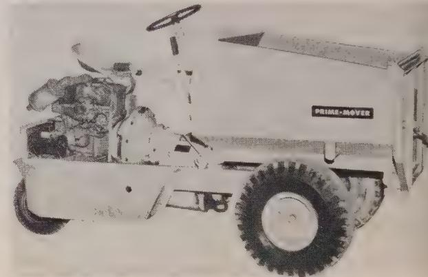
roduced to provide higher production on construction jobs by eliminating clutching and shifting and to insure quicker acceleration. The new model is powered with a Wisconsin 18-hp. air-cooled engine and a 12-volt starting system is standard. The unit can be equipped with an 18-cu. ft. dump body or a 42 x 42-in. flatbed. Control of the endgate and angle of dumping permits varying the rate of load discharge.
