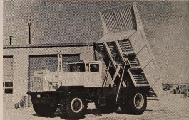
body on the new model 35SL reduces the truck weight by 2 tons and increases its capacity by corresponding amount. Truck is equipped with a 450-hp. diesel engine and a 3-speed transmission and 3-stage torque converter.
