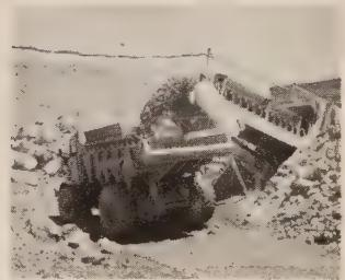
**SIERRA PIT LOADER:** Large capacity loading conveyor for materials from fine to 20" minus. Portable with exclusive "duo-belt" feature for longer belt life. Sizes from 36" to 72" belt.
