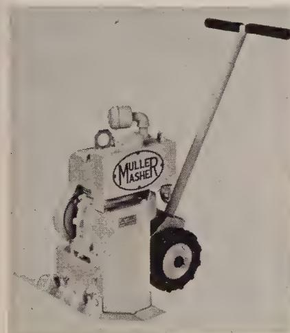
by Muller Machinery Co., Inc. The machine is self-propelled and is designed for one-man operation. It is powered by a heavy-duty engine with Stellite valve and its large eccentric weighted rotor delivers a compacting force equal to a 10-ton roller. It travels at speeds of 50 to 75 ft. per minute. Tamping shoes available include widths of 12, 18, and 24 in.
