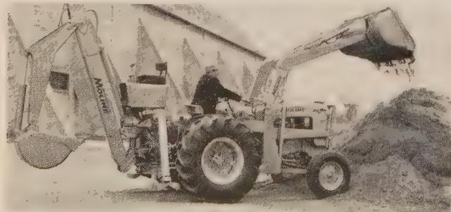
on gasoline at 2,000 rpm. Both units have heavy-duty axles and frame to handle all construction attachments, including dozers, crane hooks, mowers, back-
