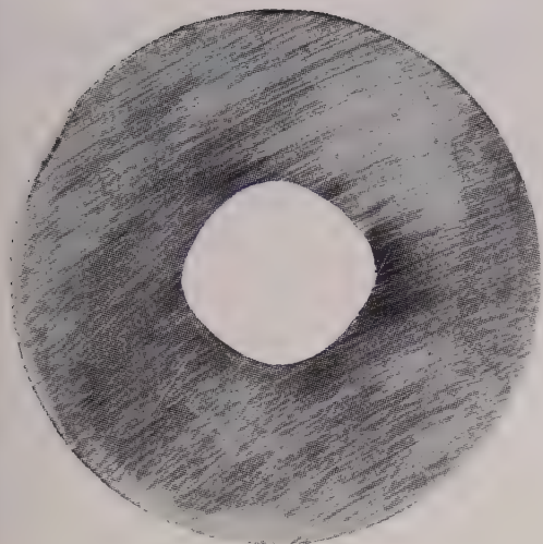
Cross section of average extension steel, showing distorted center hole.
