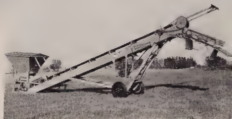
This complete Model 202 includes single deck screen, power unit, head pulley clutch and Feeder-Hopper for "top feeding" with shovel, dragline or loader.
