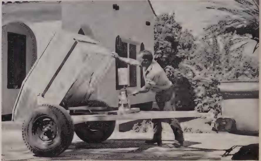
TRAILER shown in dump position, has special mechanical device for unloading. One-yard capacity unit supplies ready-mix for small jobs. Drawbar attaches to bumper.
