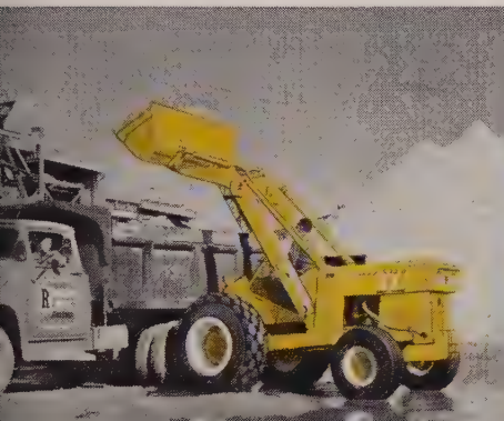
Massey-Ferguson 1001 Tractor Shovel works circles around larger, more expensive equipment. Features Instant Reverse, torque converter, direct thrust, and telescopic reach. Has large selection of attachments.
