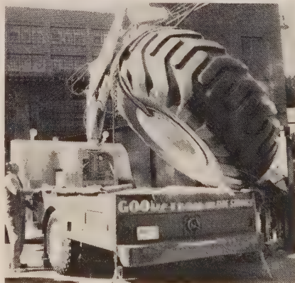
BIG TIRE SERVICE TRUCK HANDLING this rubber giant, which stands 10 ft. high and weighs nearly three tons, becomes a relatively simple task with the new "big tire" truck. E. C. Shoman of Goodyear's highway transportation department demonstrates how one man can operate the equipment, designed by George Body & Trailer Co. The tire, which is the world's largest and contains enough rubber for over 300 passenger car tires, was produced by Goodyear for earth-moving equipment. The new truck is custom built and mounted on a chassis of the four-wheel-drive type.
