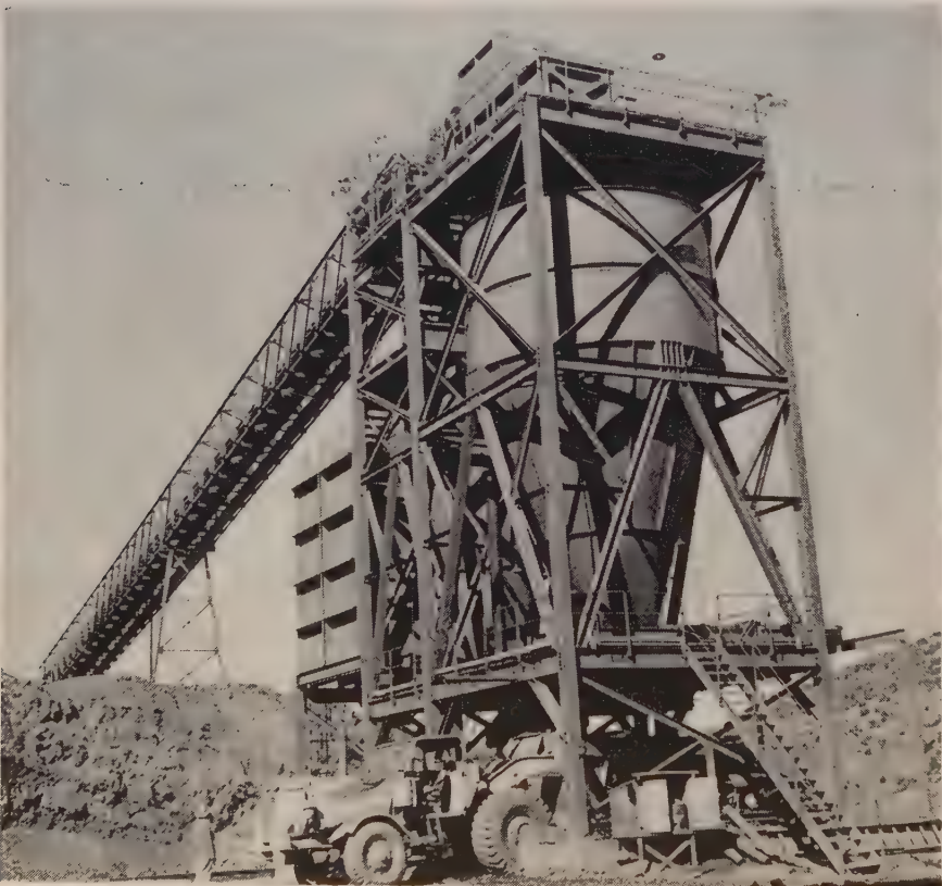
STORAGE at the end of the belt provides capacity of 2,000 yd. or about a 1-hr. run of the belt. Discharge into the fleet of bottom-dump Eucs passes through a sprinkler system that adds the required amount of moisture.
