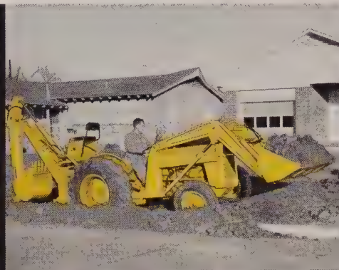
The Massey-Ferguson 204 with power-matched loader and backhoe is an outstanding performer. The 204 is the only 40-h. p. industrial tractor with Instant Reverse and torque converter; permits fast maneuverability in close quarters.
