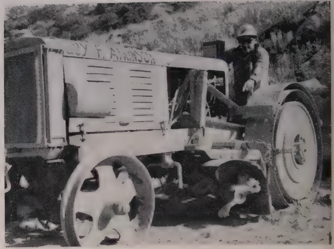
MODERNIZED Formgrader has hydraulic steering and elevation, and automatic controls. Fork, right, follows grade wire controlling depth.
