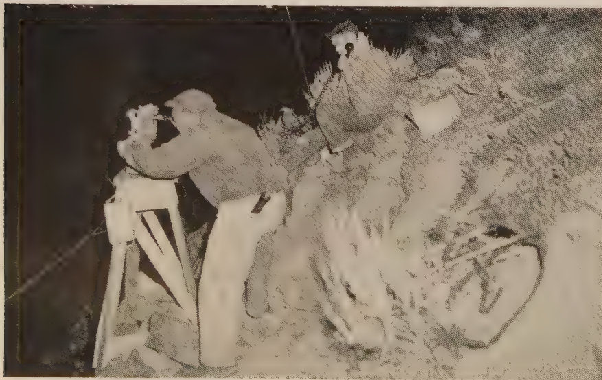
TURNING ANGLES at night on a high mountain peak with a T-3 Wilde Theodolite. Many nights, even in midsummer, the party would have to wait for hours for the icy wind to subside before readings could be made. Curious mountain sheep provided entertainment.
