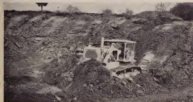
50% more production! D9E, owned by Carmichael Coal Co. near Calumet, Alabama, removes overburden of shale, sandstone and clay to uncover 30" coal seam. Coal production is 9000 tons a month.
