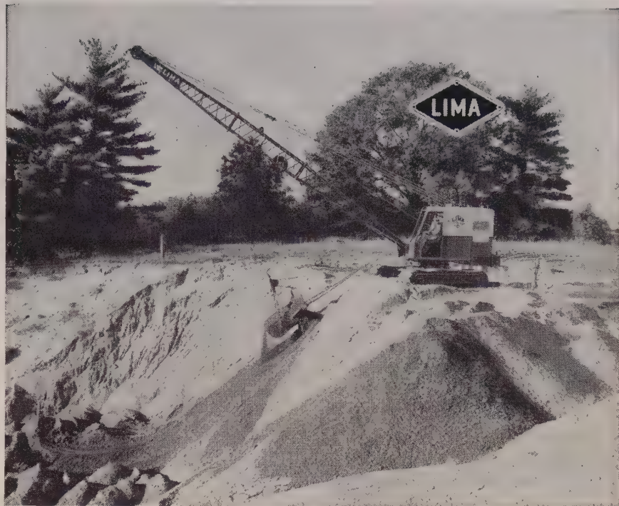
3/4-yd. Lima Type 24 Dragline handles fast and easily digging sand and gravel to feed crusher.
