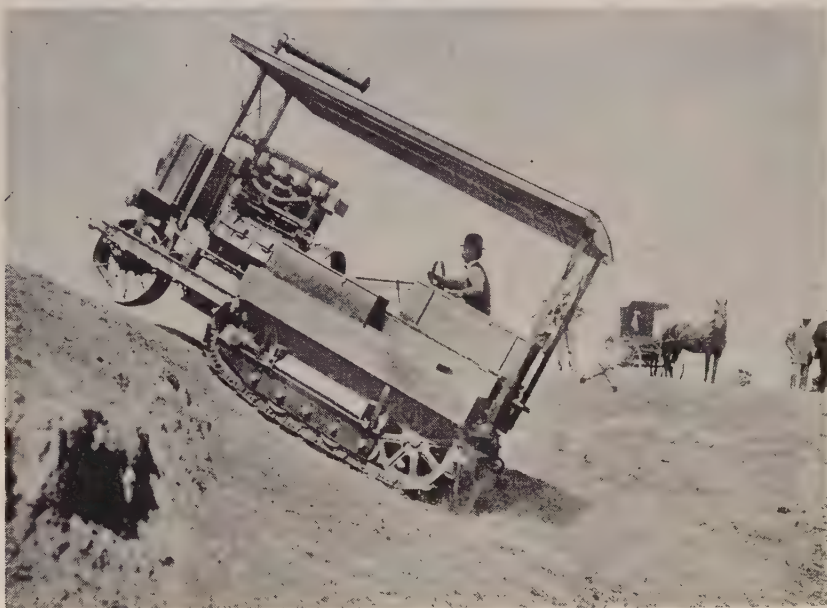
FORERUNNER of Caterpillar tractor line is this 1906 gasoline-powered vehicle, the second one built by Holt Mfg. Co., shown being tested near Stockton, Calif.
