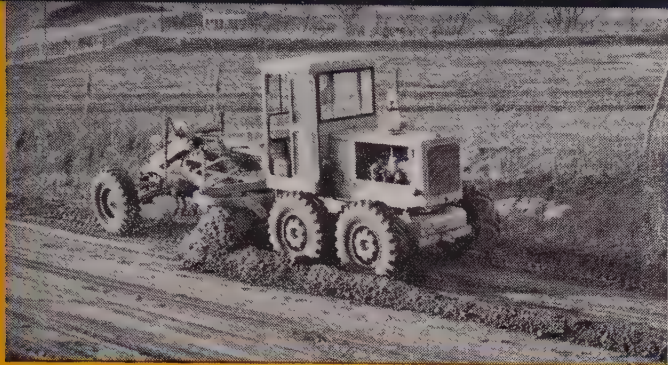
New No. 12E Motor Grader features new compact 115 HP Engine
