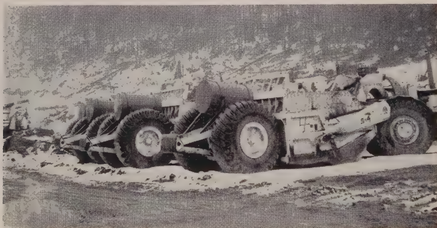
WATER DRUMS mounted on scrapers are part of sprinkling system used to cool brake housings which heated up excessively on run down steep haul road from borrow pit to river bottom.
