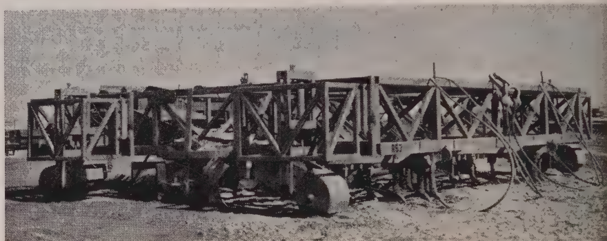
DOUBLE-windrow former used to pick up and proportion soil into windrows. Machine rides on the leaders, and is pulled by a tractor. Note plow-like ripper teeth.
