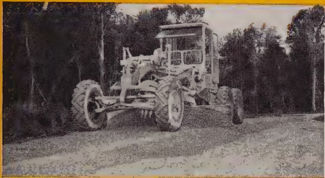
New No. 112E Motor Grader features new compact 85 HP Engine
