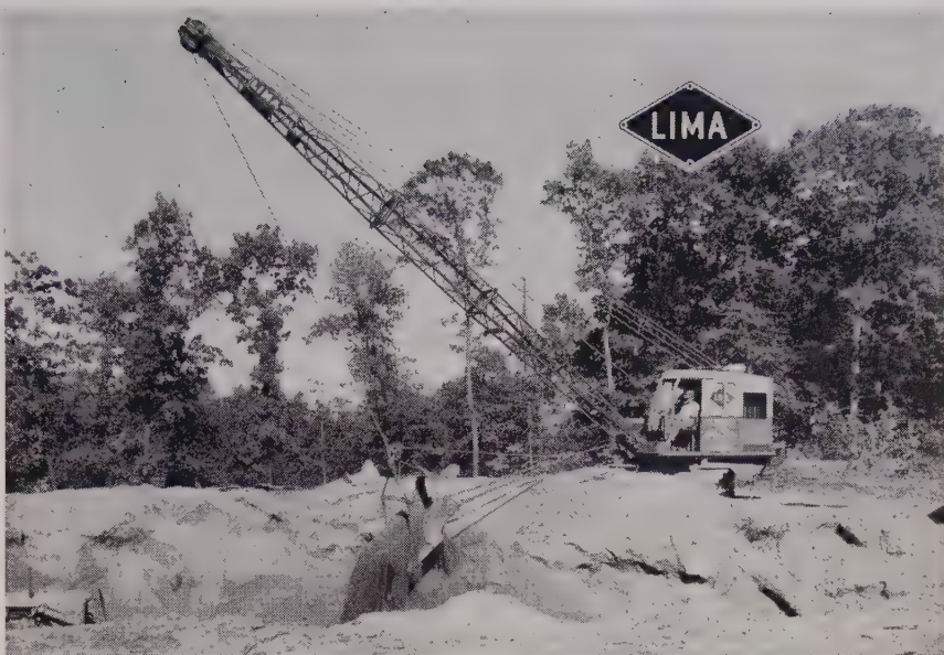
Diesel-powered Lima Type 44 Dragline speeds sand and gravel loading operations at crusher plant site in southern Michigan.
