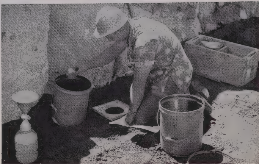
POURING calibrated sand in a completed density-in-place test hole for volumetric determination with the large sand cone. This test is being made in Zone 7 and the density plate was set 1 ft. below the surface as was done in all tests of this zone which had been compacted by sheepsfoot roller.
