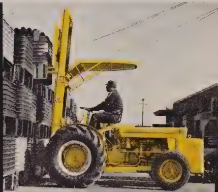
The Massey-Ferguson 204 Fork Lift—newest in the Massey-Ferguson line with "Instant Reverse." Has 5000 pounds capacity. Numerous attachments, including 20' mast extension.
