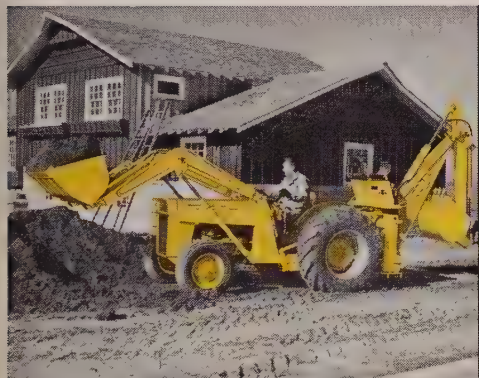
The Massey-Ferguson 204, 40-h. p. Industrial Tractor with matched Loader and Backhoe. Also has "Instant Reverse" and torque converter for faster work and maneuverability in tight areas.
