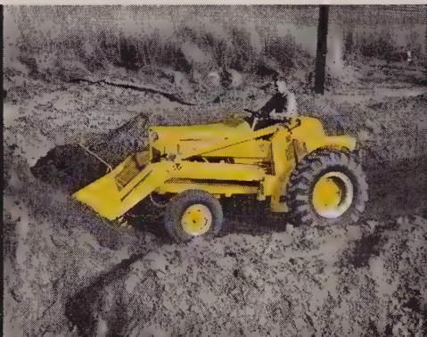
The Massey-Ferguson 406 Tractor Shovel. 1 cu. yd. (SAE rated) capacity. Has "Instant Reverse," torque converter, rear-wheel drive. Multiple attachments for low-cost versatility.
