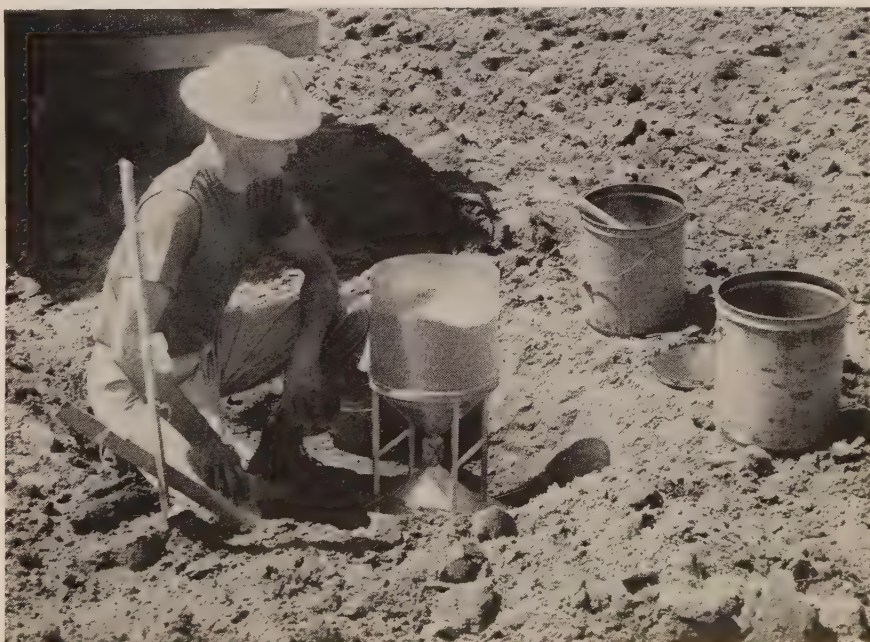
MAKING a density-in-place test at one of the dam abutments in Zone 7. Soil is being carefully removed from the hole and placed in the 5-gal. paint pail which has a clamp type lid to seal in the moisture during transportation to the laboratory. Volumetric measurement will be made using the small sand cone shown with its previously weighed and calibrated supply of sand.
