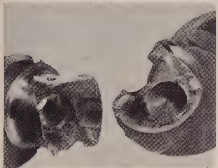
TORSIONAL vibration fracture characterized by a break at a 45-deg. angle, usually toward rear of engine.
