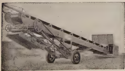
Single-deck vibrating screen folds into towing position for transportation without dismounting screen or removing any of the drive assembly.
