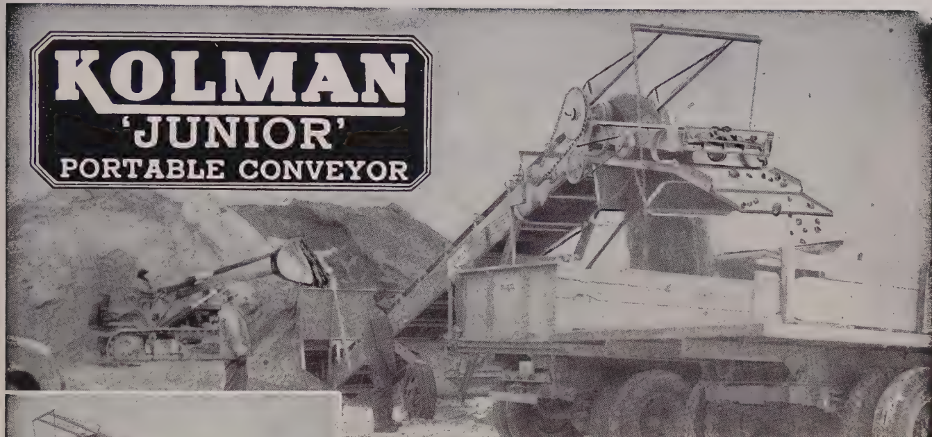
Loading sand and gravel is easy for the City of Yankton, S. D., with their new Model 202 Kolman Junior conveyor-screen plant. 40 feet long and with a 24" belt, equipped with a Kolman SB-60 vibrating screen, 6' x 36".
