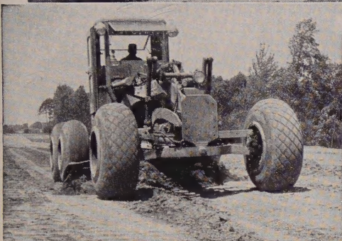
MICHIGAN —T-600 Grade-O-Matic Grader with sand tires on Route #12 near Battle Creek.
