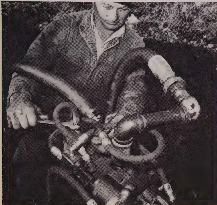
Aeroquip Hose Lines, with Reusable Fittings, completely replaced copper tubing formerly used as feeder lines on Emsco stomper.
