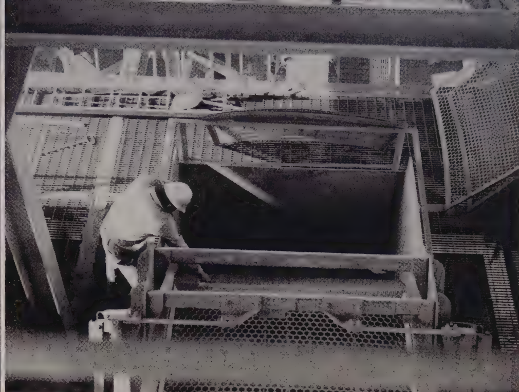
◀ Left: Close-up of Amsco Chute Plates used on each discharge Hi-G screen. Right: General view of Hi-G screen in screen house of large New England quarry. ▶
