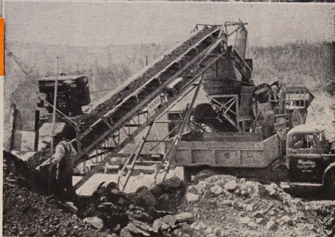
50-ft. Kolman Model 101 with 36" belt shown separating fines on Hopkins Construction Ltd. job near Edmonton, Alta. Equipped with Model S8-80 Kolman single-deck screen and feeder-trap combination.
