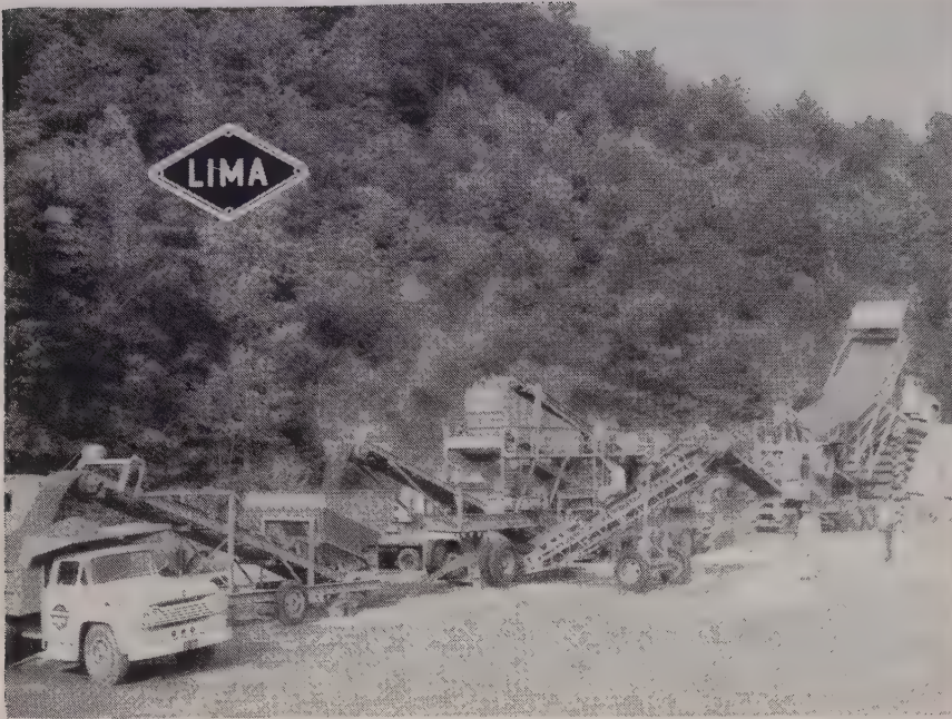
Completely portable Lima A-W crushing installation has primary 20 by 36-in. jaw crusher, Model 101-CE secondary plant and 7-yd. surge bin. Delivers exceptionally high production for Maymead Lime Co. in Tennessee.
