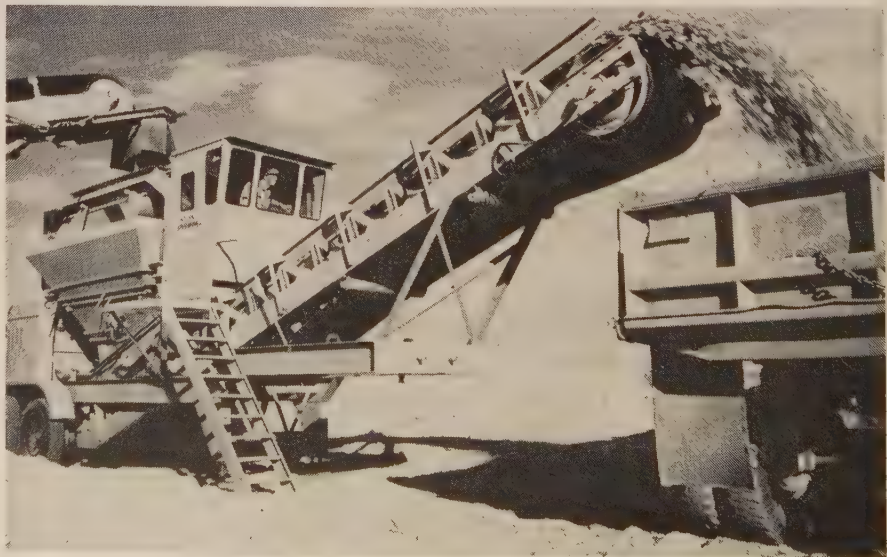
ELECTRONIC scale-loader handles a 6-ton batch in 30 seconds. Unit developed by Idaho firm uses "load-cells" instead of levers to determine weight.
