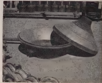
CRUSHER parts faced with chromium cast iron
