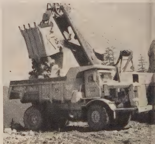
Six 27-ton and two 22-ton Rear-Dump "Eucs" haul rock from the quarry to the fill... all of these units are equipped with Torqmatic Drives and Torqmatic Brakes.
