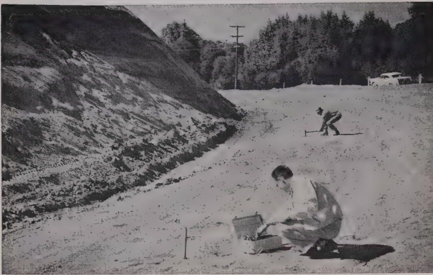
FAST and simple is the equipment and procedure adapted by Caterpillar Tractor Co. Shock waves produced by sledge hammer on a steel plate are timed by the instrument and can be interpreted to indicate rock conditions to depths of 50 ft.
