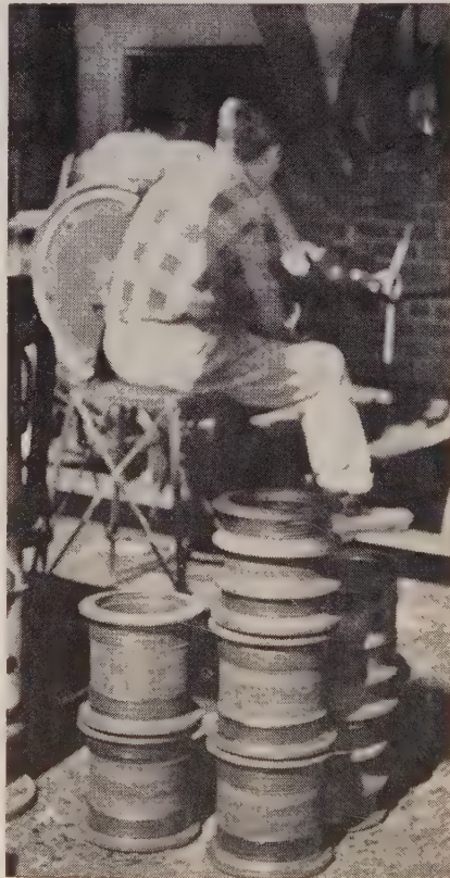
TRACTOR rollers faced with chromium steel
