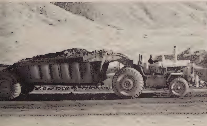
Big loads of heavy gravel move over good haul roads at fast travel speed in these Bottom-Dump "Eucs". Torqmatic Drive — torque converter and semi-automatic transmission — provides full-power shift and a smooth flow of power to meet all road and grade conditions on the 5 mile cycle.
