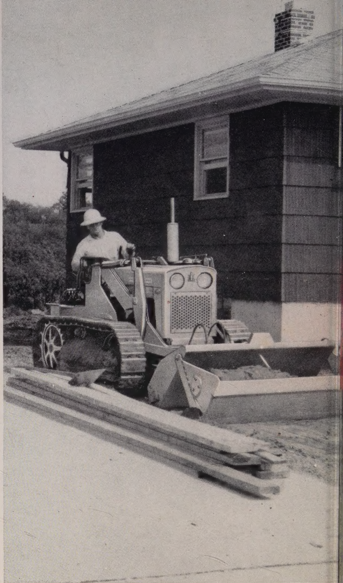
The exclusive International Drott 4-in-1 combines standard \frac{3}{4} cu yd bucket, plus clamshell (shown), carry-scraper, and bulldozer, all in one machine.
