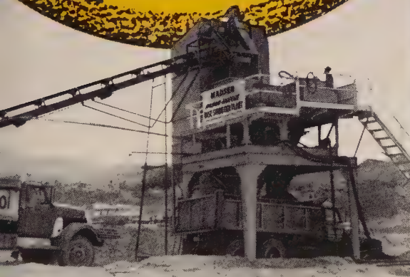
MADSEN HIGHWAY-AIRPORT BASE STABILIZER PLANT ...newest addition to the MADSEN line. This plant is a high-production, portable unit designed specifically to meet today's exacting requirements in regard to precision proportioning and control of materials. The twin-shaft continuous-type pug mill mixer is designed for producing 600 T.P.H. of stabilized mix. Plant features rugged construction, mechanical simplicity and easy maintenance.
