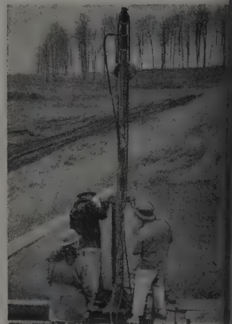
A Sprague & Henwood crew recovering a 30 foot sample of sensitive marine clay.
