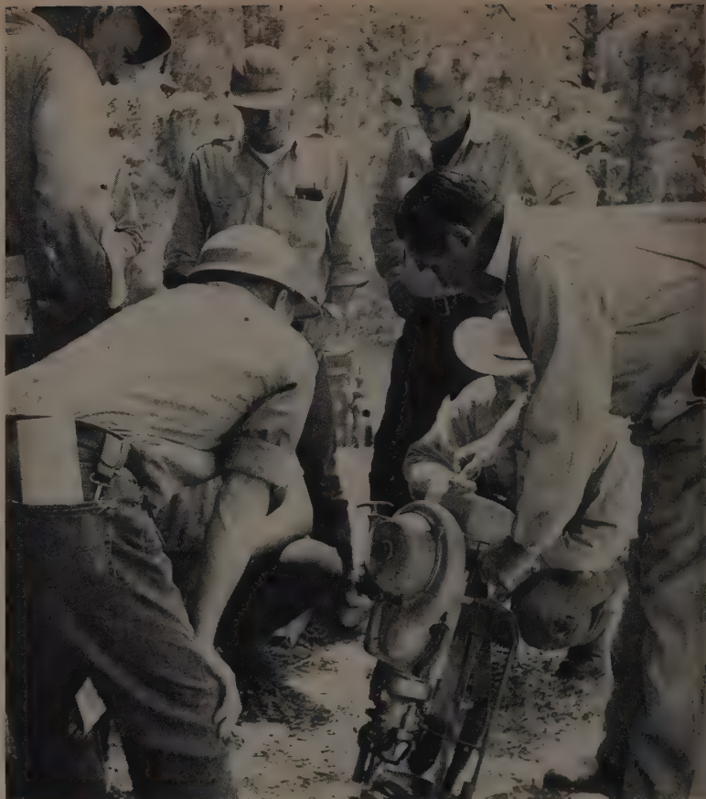
FOREST SERVICE personnel watch a demonstration of the light, self-contained, gas-powered drill. Drilling position can vary up to 45 deg. Pulley-type starter is visible in photo.
