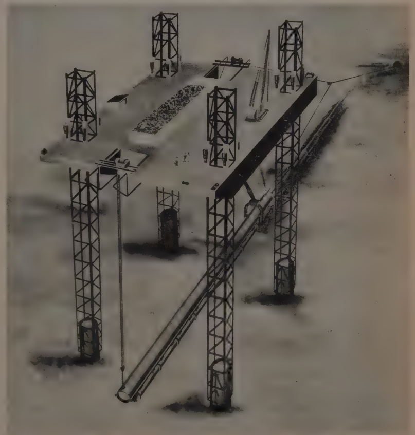
SIMPLIFIED DRAWING shows how floating platform operates. Jacks lower legs to ocean floor and elevate platform above water to free it from influence of waves. Pontoon-strongback with 192-ft. long string of pipe is floated into position underneath platform. Water is admitted into pontoon and cables lower it into trench. In-haul cable pulls pipe into joint. Rock ballast is placed through telescoping tube from bins on platform to split tremie tube (visible in drawing) which rides rails on pontoon. TV monitors operation. Full details are given in text. For photograph of platform see front cover.
