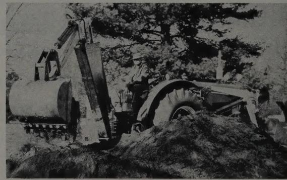
diesel or LP gas engines. Equipped with International Wagner or Pippin backhoe with 14½-ft. working depth, the unit also is designed to work with Wagner ¾-yd. front-end loader, and four models of the Johnson elevating scraper with 4 to 8-yd. capacities. Pulling power of the 660 with sheepsfoot rollers is said to equal crawler units of 100-hp. class. The new tractor has a road speed of 16.5 mph., with attachments.
