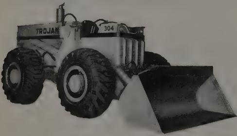
New low silhouette for greater visibility. Exceptional service accessibility . . . Heavy-duty front bumper integral with frame for added protection . . . Recessed headlights . . . 24-volt starting and lighting system . . . Foam rubber bucket seat for operator comfort.
