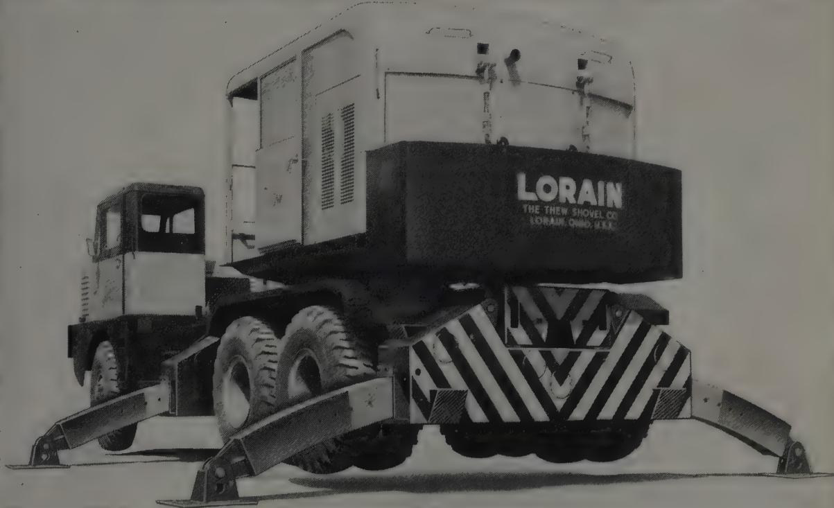
Full operation with wheels off the ground . . . proof of how two wedge locks hold beams so securely that you can operate at full rated capacities. Off-the-ground jacking ability is good for quick tire changes or for lifting out of soft spots.
