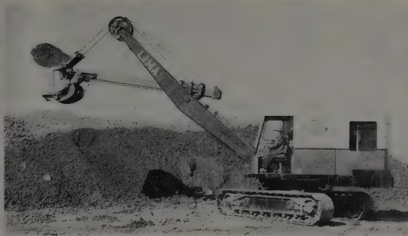
**NEW POWER SHOVEL, Type 64, recently introduced by Baldwin-Lima-Hamilton Corp., has a 1 1/4-yd. dipper on 17-ft. handle and 20-ft. boom. Equipped as a crane it has a capacity of 40 tons. New model offers two sizes of crawlers, both demountable for highway transport. Special heavy-duty version, Type 64 SC, has 50-ton capacity and power features for special jobs.**
