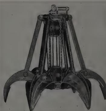
field tested rip-rap handler is designed to pick up stones easily and is adapted specially to the unloading of gondola cars. In the  $\frac{1}{2}$ -yd. size the bucket weighs about 2,000 lb. and the large size 2-yd. bucket weighs 12,000 lb.
