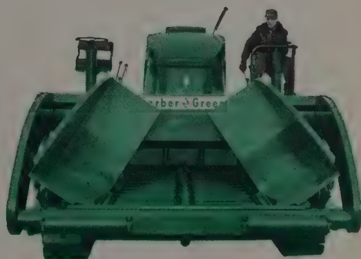
Self-cleaning, hydraulically operated hopper extends to extreme rear of chassis where gates are located.
