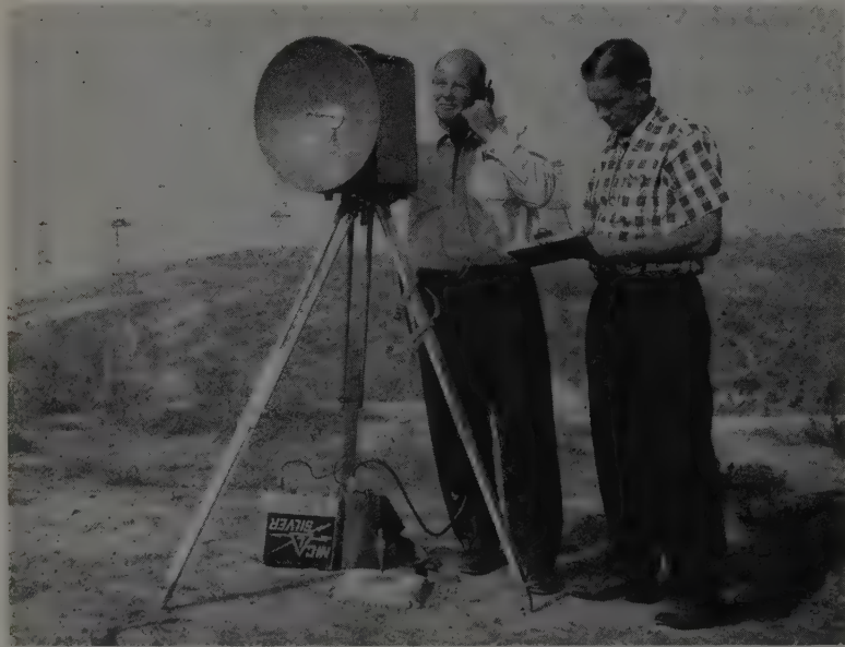
CALLING OFF readings from the instrument panel of the Tellurometer is Dick Estabrook, chief of surveys, Orange County, while Owen Vineyard, deputy county surveyor, takes notes. The new system of surveying is being used to speed up a county-wide mapping program. About 10 to 15 min. are required to unpack and set up this master unit over a known point (note plumb bob) while the remote unit is set up at a point to be observed. Only 10 min. are required to obtain the measurement.
