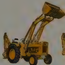
Work Bull 303 with 500 Loader and Dams Backhoe
