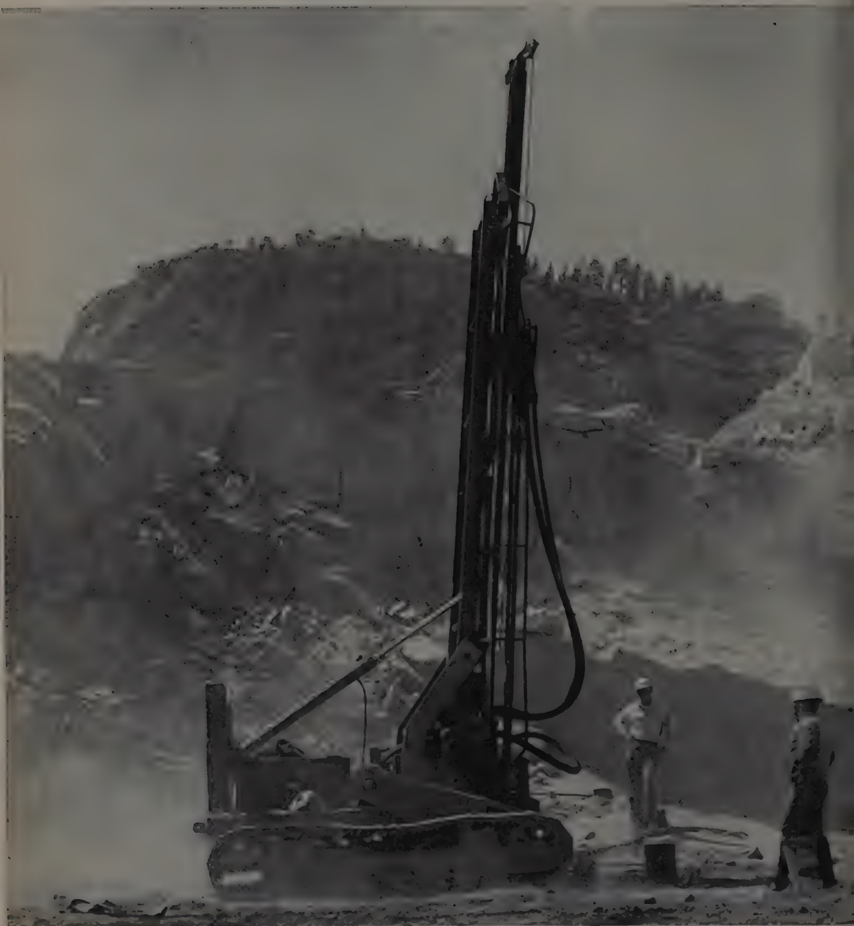
A 5½" hammer wallop. Here's deep hole drilling power in a class by itself. Gardner-Denver DH143 fills the rock drill gap between wagon drill and rotary rig.
