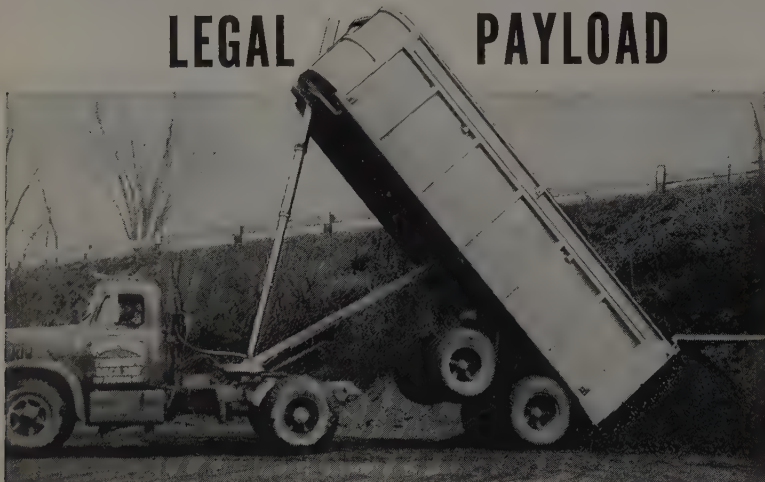
This 28 yard aluminum frameless dump trailer is shown stock-piling coal. It is equipped with F-714-T-156 front end hoist.
