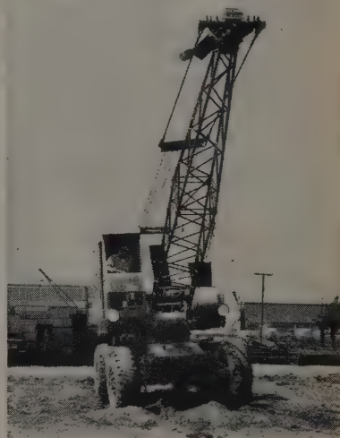
Notice how wheels on the oscillating, spring-mounted front axle of the SP-107 hug the rough terrain ... keep powerful, 4-wheel traction at work.
