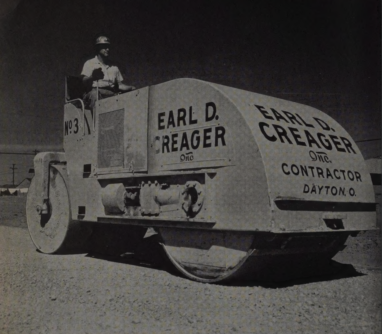
A-W Tandem Roller compacting base for asphalt road at Dayton, Ohio. Owned by Earl D. Creager, Inc.
