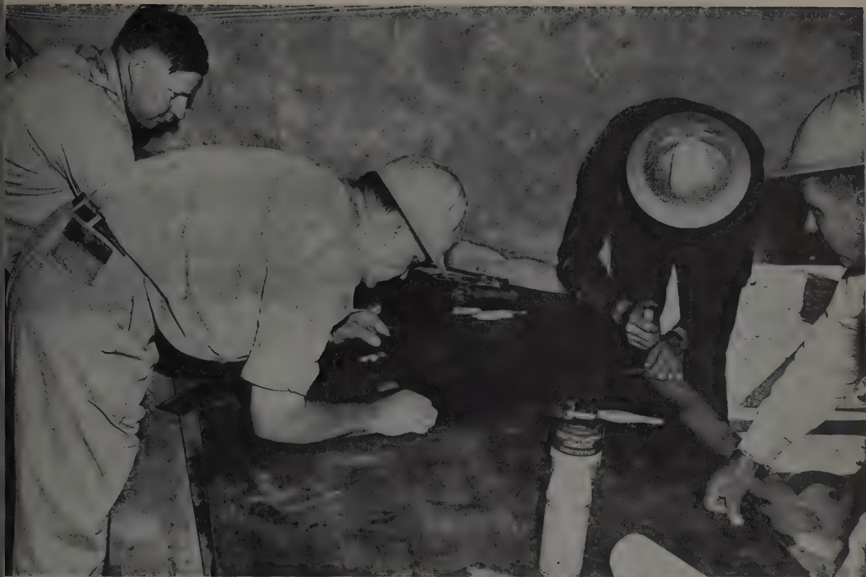
SPlicing the 42-in. wide belt takes skill and patience. A portable electric cookstand which completely covers the belt does the final
