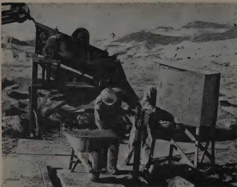
MATERIAL BROUGHT up by the bucket drill was moved by belt conveyor to an Overstrom double-deck screen. Four sizes were chuted directly into wheelbarrows and weighed. Weights of fractions were obtained for each foot of hole. The minus \frac{3}{4} -in. size was analyzed further.
