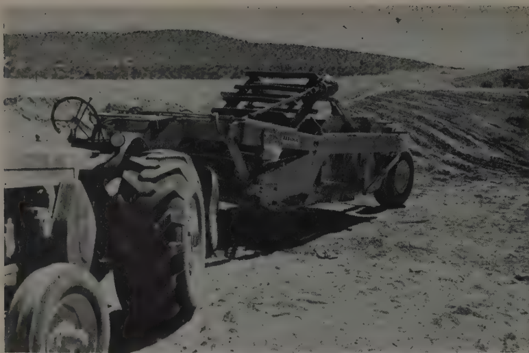
FINISH GRADING is done with Cat No. 12s followed by pictured light scraper which loads by means of a conveyor. Rig is pulled by John Deere industrial wheel tractor.
