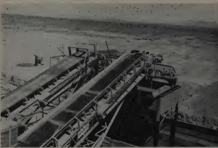
TWIN KOLMAN LOADERS in base material pit will produce at a tremendous rate. One man located between belts will control speeds of both belts and both surge hopper gates. Vibrating screens will shunt oversize to Pioneer crusher now being assembled.
