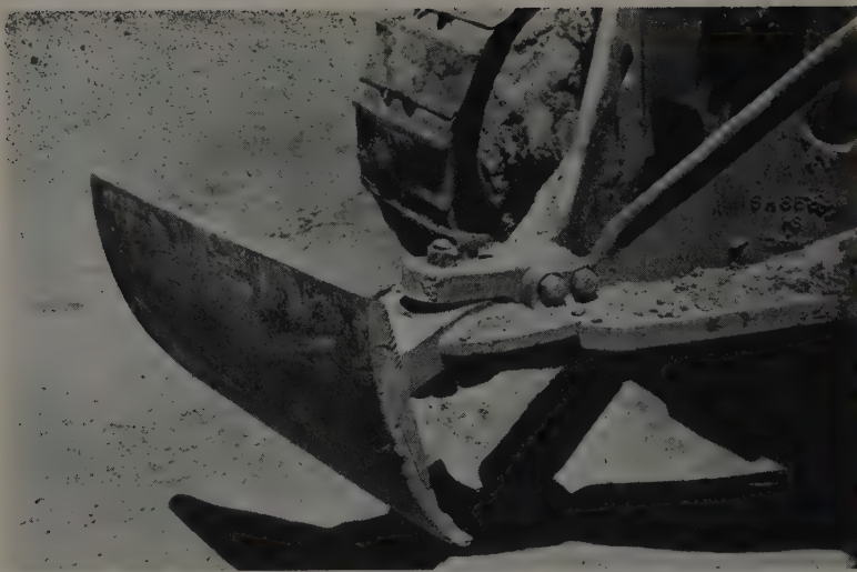
PUSH PLATE on rear of Cat D9 used for tandem pushing of scrapers is product of Shepherd Machinery Co. Skilled operators keep contact shocks low during loading without time loss.
