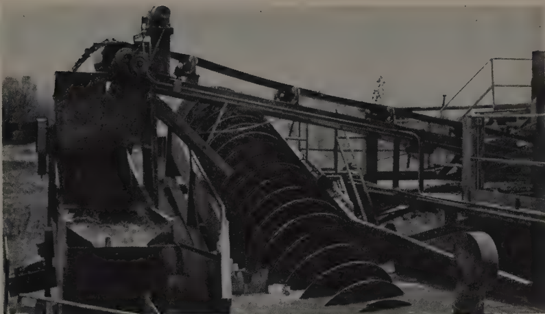
PAVING AGGREGATE at the Monarch plant is shown going through a Wemco sand washer and classifier, with the rock going through an Eagle Iron Works washer. After another screening the sand is re-washed before going to stockpiles for dewatering.
