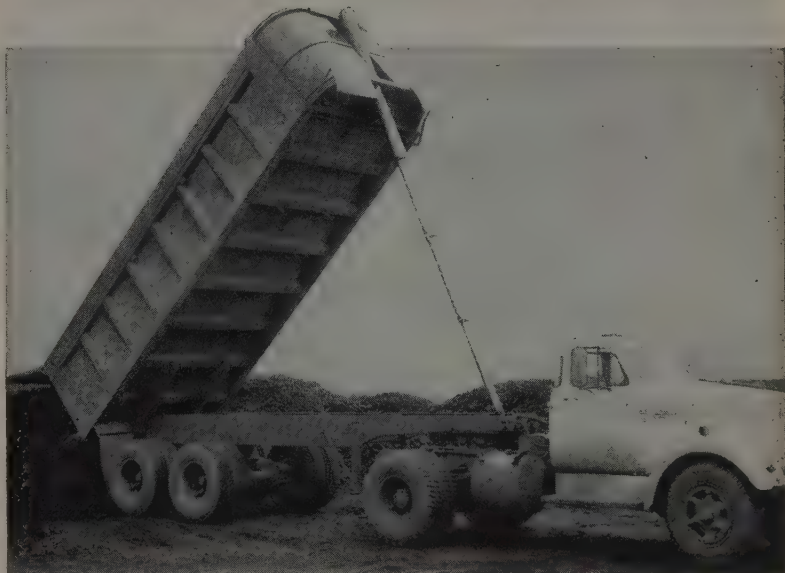
This 27-yard body with F-715-T-204 front end hoist is dumping a 44,000-pound load of coal in six-foot high stockpiles.
