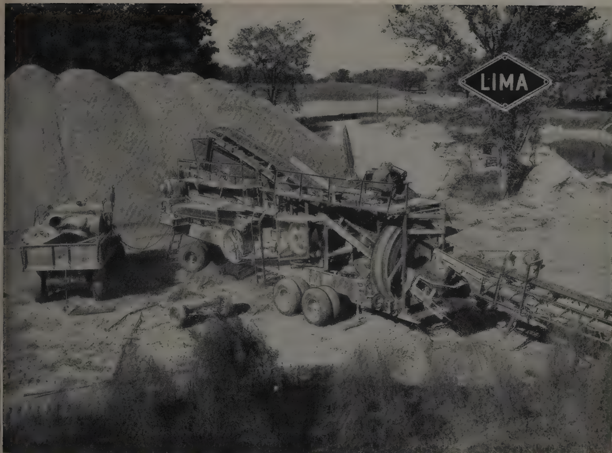
Lima Austin-Western 111 Crushing and Screening Plant, owned by Ronald Weaver, Dansville, Mich. High-grade specification material is being produced at an average rate of 1000 cu. yd. per 9 hr. shift.
