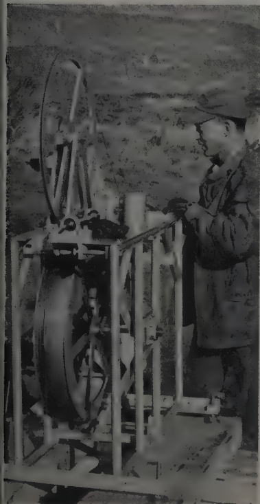
LOWERING device at John Day location. The pay-out reel has 500 ft. of camera cable. Passing over the upper reel it automatically controls the electrical circuits for flash and camera drive.
