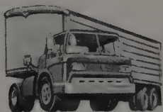
New Ford C-1000 with the 260-hp. 477 Super Duty V-8 engine. Maximum GVW 31,000 lb., GCW 65,000 lb.
