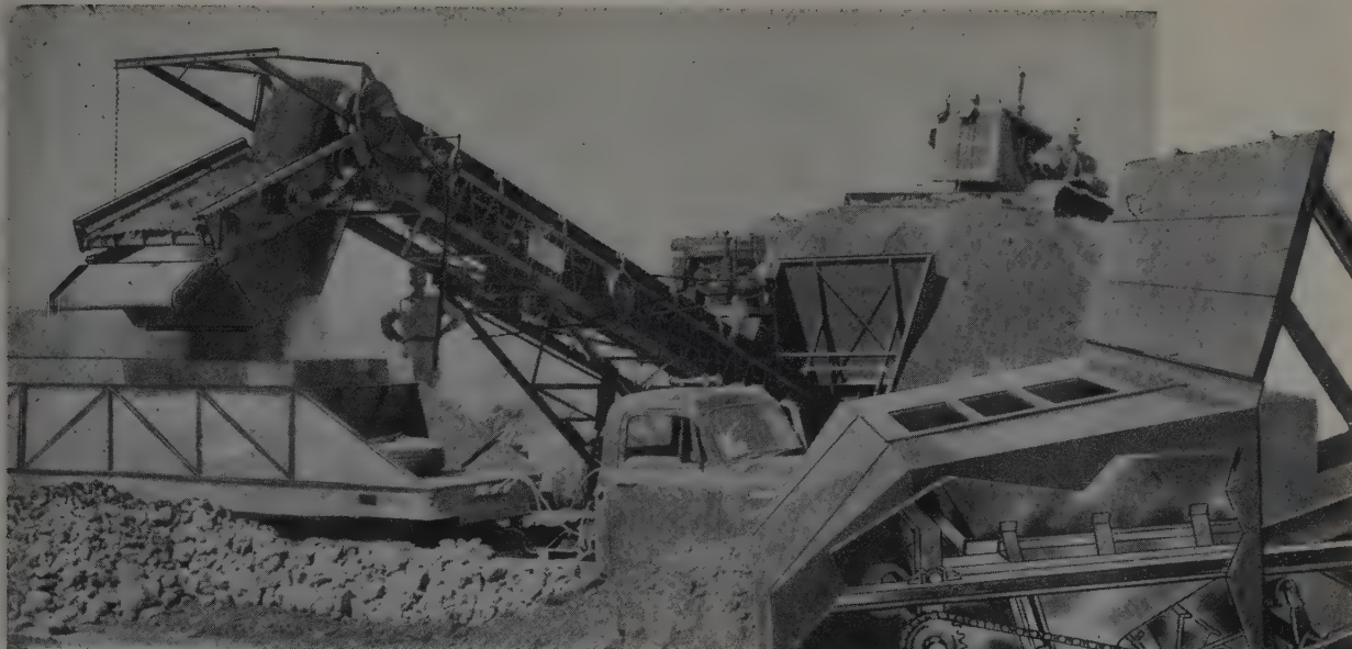
Above, 50' x 36" KOLMAN Portable Conveyor-Screen Plant equipped with built-in feeder and wing wall. Owned by Peter Kiewit Sons' Co.
