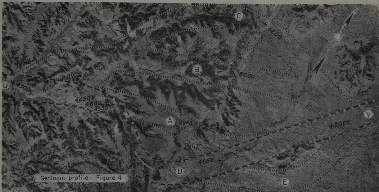
FIG. 3. A small scale uncontrolled mosaic indicating the five main route bands, A, B, C, D, and E. Boundaries of abandoned alternatives are shown with dotted lines, and boundaries of best route in dashed lines. Air line distance between control points U and V is 9½ mi.
