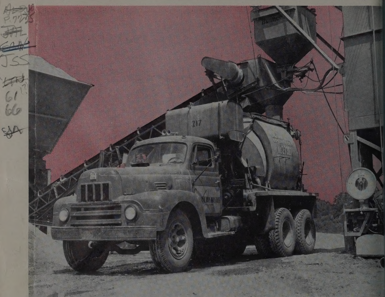
One of the Heston fleet—an International L-190 with RD-406 engine, equipped with a 5-speed Fuller 5-A-62 Transmission.
