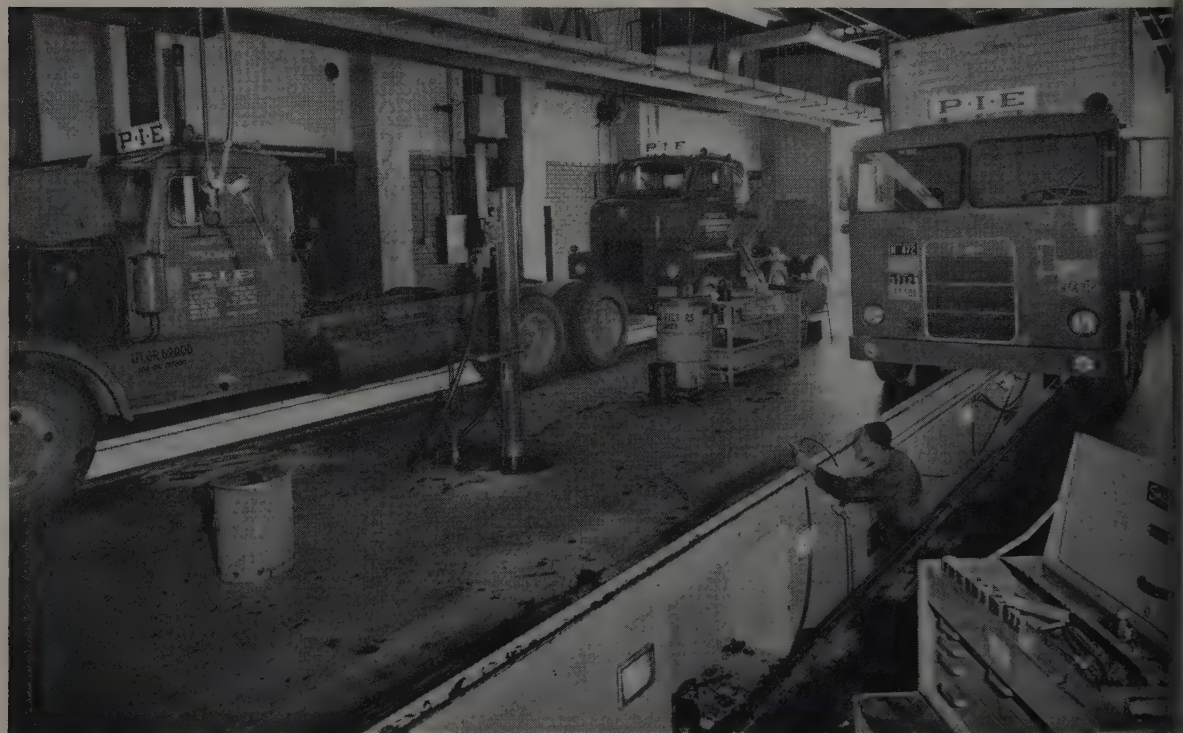
MAINTENANCE is speeded and improved with good working conditions. This is the type of head-high service pits, with adequate lighting,
