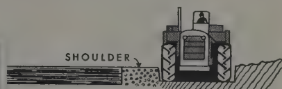
1. D Tournapull® cut flat trench 7' wide, adjacent to existing shoulder.
