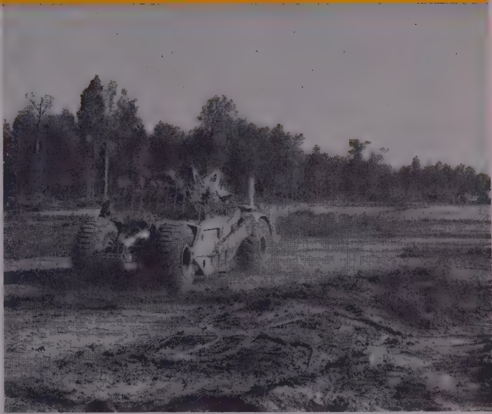
DW21-NO. 470 LOWBOWL SCRAPER speeds heaped load on haul. Turbocharged 6-cylinder Cat Engine, also in the DW20, delivers 300 HP (maximum output)—power aplenty for working in tough conditions.
