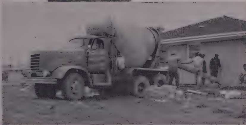
One of Rockwell Lime's fleet of FWD 6-wheel-drive ready-mix units with 10-speed Fuller 10-CB-65 Transmission.
