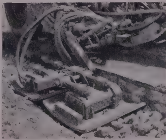
Widener Attachment —Vibrating shoes compact material in widening trench while Roadpacker runs on existing pavement. Easily adjusted for various width trenches.
