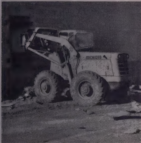
Lumber — as much as \frac{3}{4} of a truck load (3500 to 4000 lbs) unloaded at once, stockpiled, later carried to hoist.
