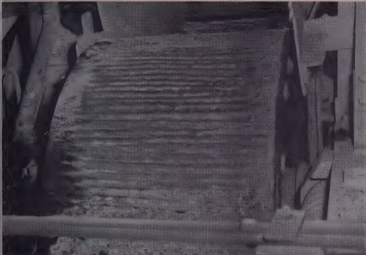
This roller, hardfaced with Victor alloy, shows practically no wear after crushing 40 tons of rock hourly, 8 hours daily for 30 days.
