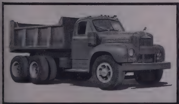
B-40 SERIES —Widely popular for maneuverability and rugged strength. B-40 four- or six-wheel dumpers, mixers, flat-bed trucks and tractors are especially valued for their bonus capacities, economy, and handling ease. Powered by Mack 150 hp Thermodyne diesel or Magnadyne gasoline engines.
