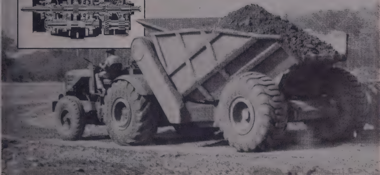
The new Wooldridge "Cobrahaul" Rear Dump Unit with Fuller 9-speed R-1150 ROADRANGER Transmission.
