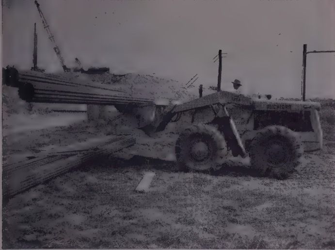
Carries pipe —One of Peter Kiewit's Michigans serves as all-around handyman on company's Indiana Turnpike contract. This 95 hp model lifts up to 11,000 lbs, carries 5,500 lbs at 4 mph. Note excellent all-around visibility given operator.
