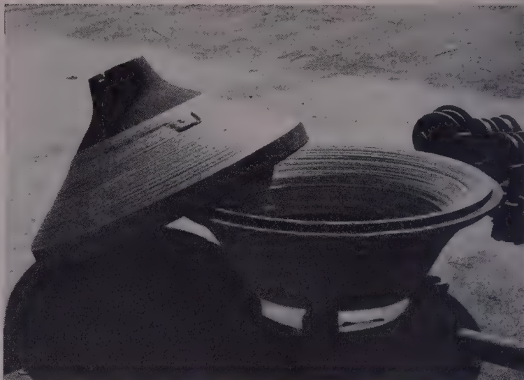
Note even deposit of Victor VA#3 automatic rod on gyrotory crusher cones.
