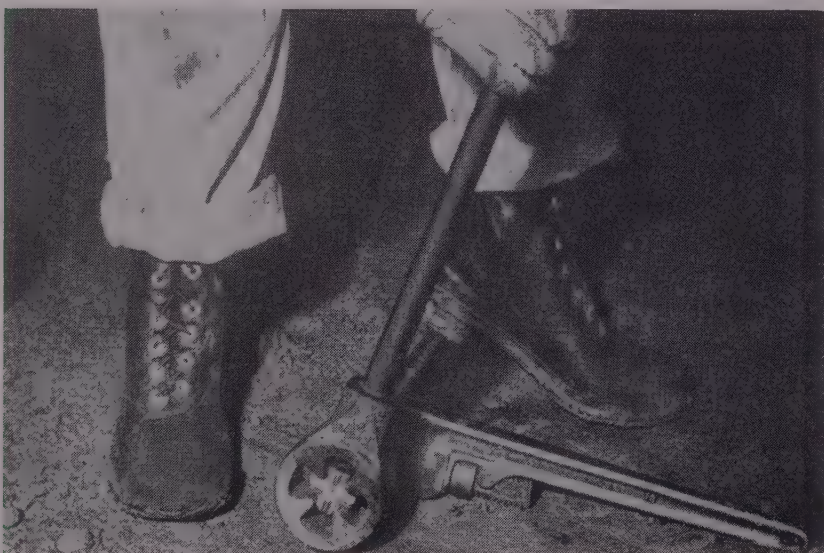
A BOX WRENCH for detaching bits cuts down damage from improper methods of removal.
