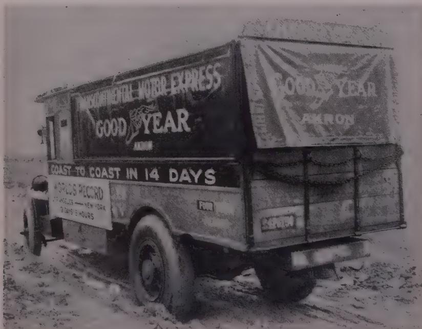
FIRST pneumatic-tired truck to carry a pay load—much of it was spare tires—in 1916. It is shown enroute from Los Angeles to New York, which required slightly less than 14 days. Years of improvement intervened before the Nylon, tubeless tire that is the truck standard of today.
