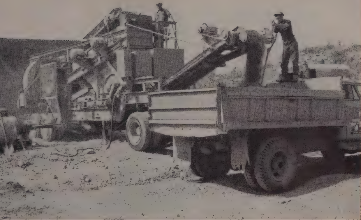
The 201-E is a highly portable plant. The frame is extra strong to hold rigid alignment of all equipment and drives. A rocker beam with full width axles supports most plant weight. Four wheels, each with dual tires, oscillate separately to compensate for rough terrain.
