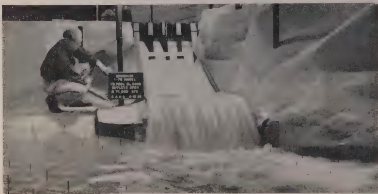
MODEL OF BROWNLEE on a scale of 1 to 70 is being studied in the hydraulics lab of the State College of Washington to determine best spillway design. Shown is a test of a flip bucket spillway. The model includes a scale replica of the streambed \frac{3}{4} of a mile above and below the dam. Dr. E. Roy Tinney is in charge of the laboratory, which also is carrying out tests on a model of Noxon Rapids Dam in Montana.
