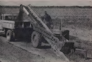
Model 550 removes windrows in a hurry... with a capacity that keeps ahead of all trucks normally available. This light, highly maneuverable machine reduces windrow loading to lowest cost. Self-propelled at 10 m.p.h., with a turning radius of 8' 6".
