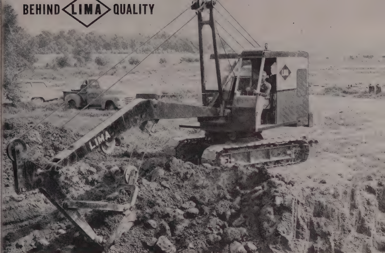
LIMA Type 24 Pullshovel with 17' 6" boom, 6' 0" bucket arm and 1/2 cu. yd. bucket.
