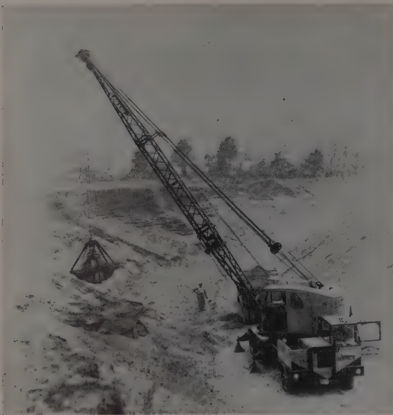
MODERN PIT-LOADING with a truck-crane of Thew-Lorain Shovel Co. emphasizes portability.
