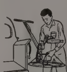
Midget Trowel. New Lightweight, one man carries; gets into tight spots; only 24" across yet does top trowel job 6 times as fast as by hand. 70 lbs.; 1.6 hp engine.
