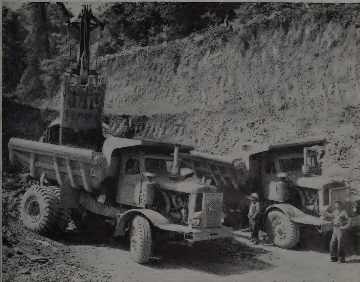
Two of the fleet of 28 Euclid 46TD 22-Ton Dump Trucks equipped with Fuller 10-F-1220 Transmissions, and operated by Nello L. Teer Company, Durham, North Carolina.
