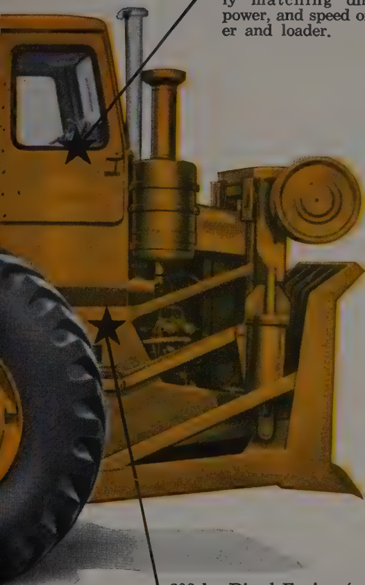
208 hp Diesel Engine (synchronized with rear engine)
