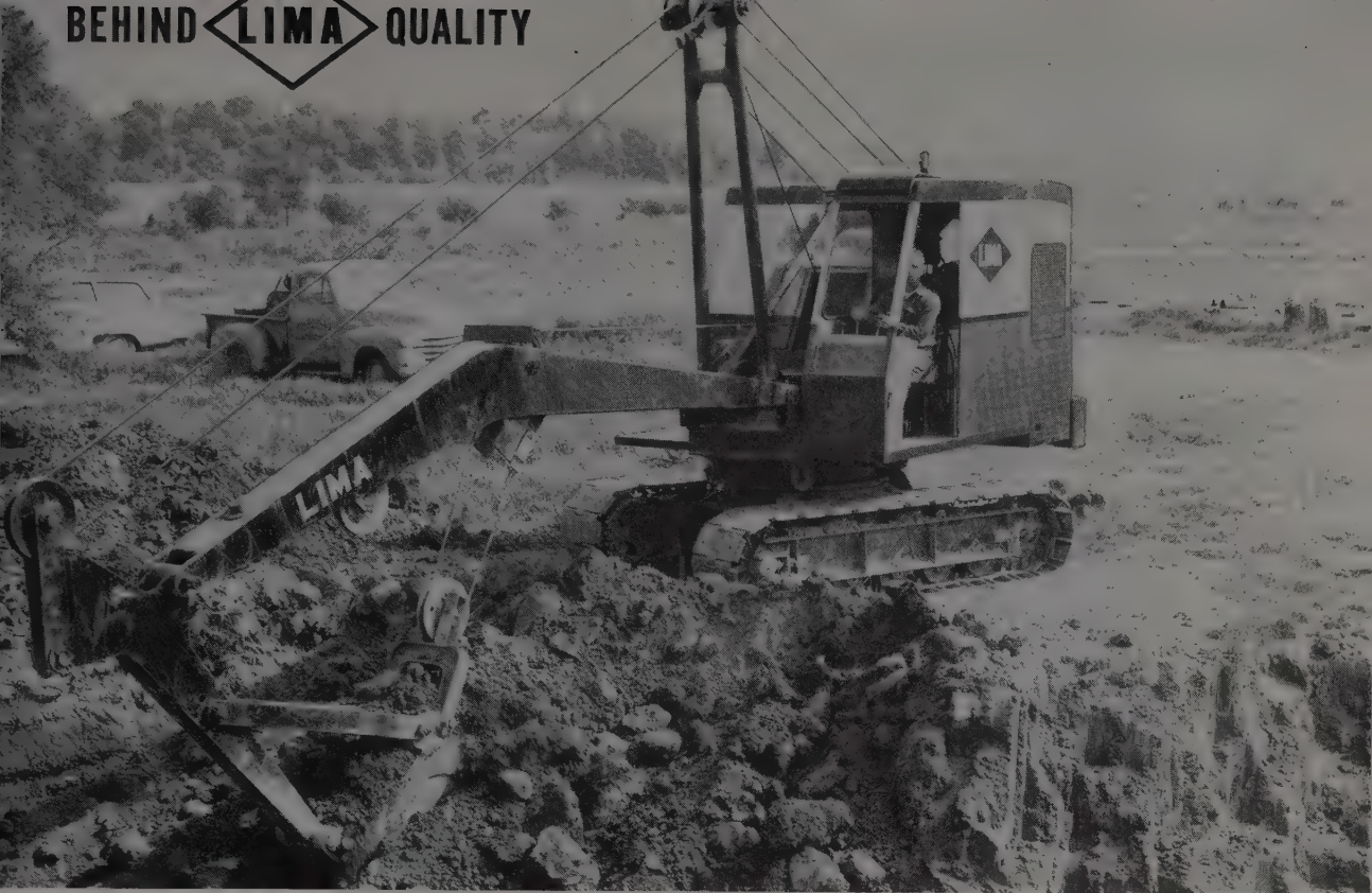
LIMA Type 24 Pullshovel with 17' 6" boom, 6' 0" bucket arm and 1/2 cu. yd. bucket.
