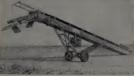
Complete plant is compact unit for big production, convenience of operation, ease of transportation. Rugged enough to carry a loading trap and large vibrating screen without additional support.
