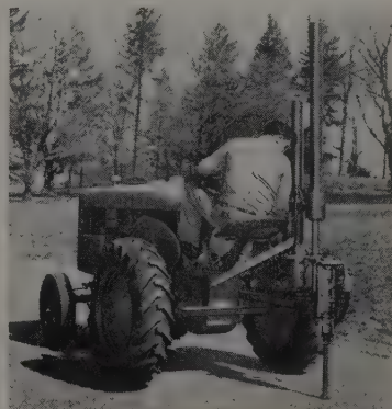
Pneumajack, mounted on a Standard Pneumatractor, does a variety of jobs from drilling for mud jacking to production drilling.
