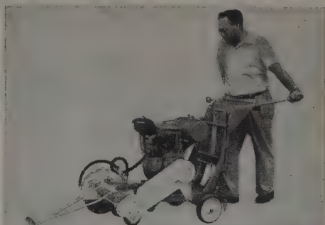
1 FELKER MODEL 100 —A low priced concrete cutter for patchwork and light cutting. Light, exceptionally maneuverable. 7.5 hp Wisconsin drives 8" through 12" blades. Right or left hand operation with double end spindle.
