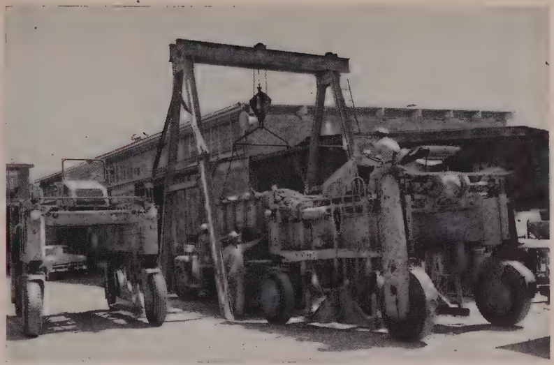
ARRIVING at the yard the full container is set down under the A-frame, and the carrier picks up an empty and heads for the next collection job. Clementina makes 40 to 50 runs a day.
