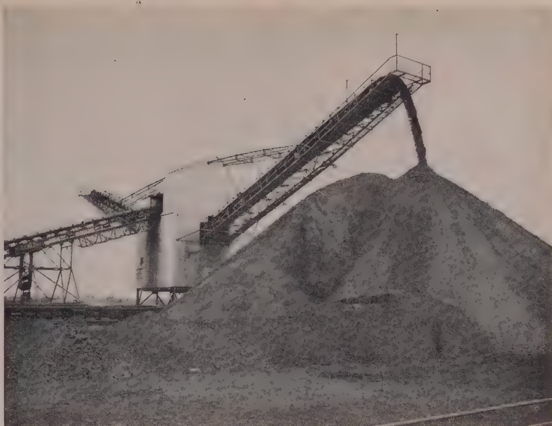
The S-A Conveying System provides for stockpiling or loading at dockside. Here, the traveling stacker is building a stockpile at the rate of 3750 net tons per hour. Conveyor booms stockpile to either side.
