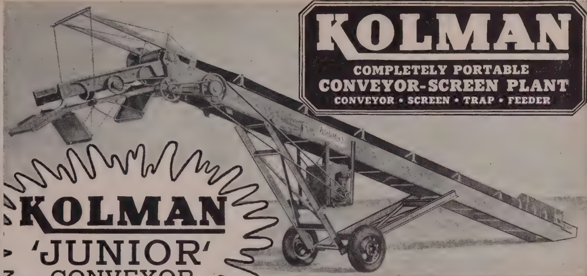
KOLMAN Model Junior Conveyor 40'x24" with gasoline engine and 6'x36" Model SB-60 Kolman Vibrating Screen
